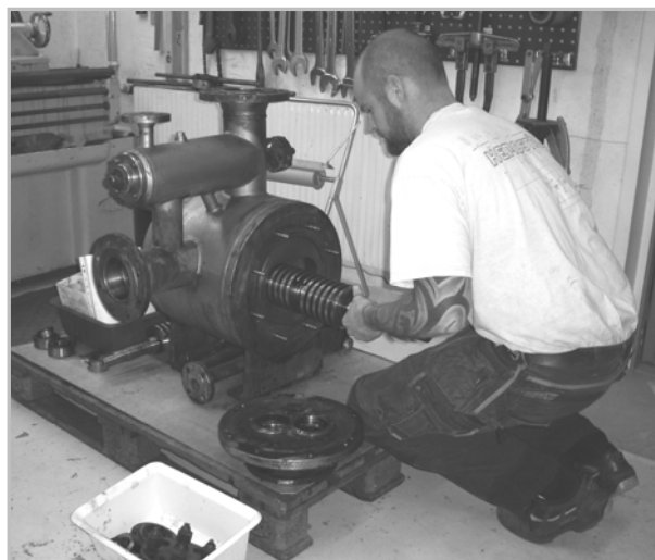
Bornemann W5.2zk-20 under reparation
